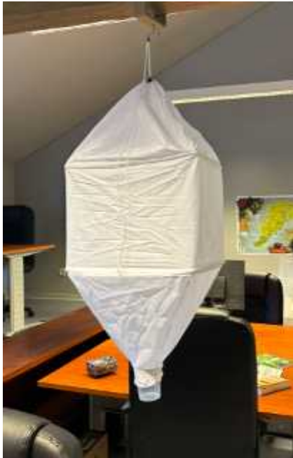
A Winkler extractor bag with collection cup tied below.
