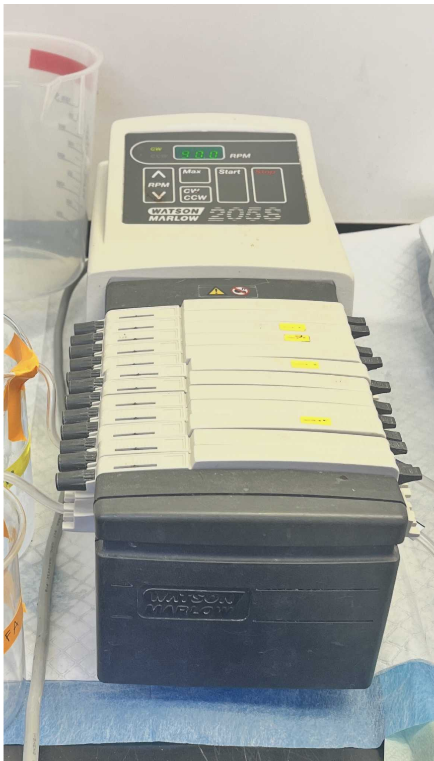
Closer look at peristaltic pump with y-shaped tubing threaded into cassettes.
