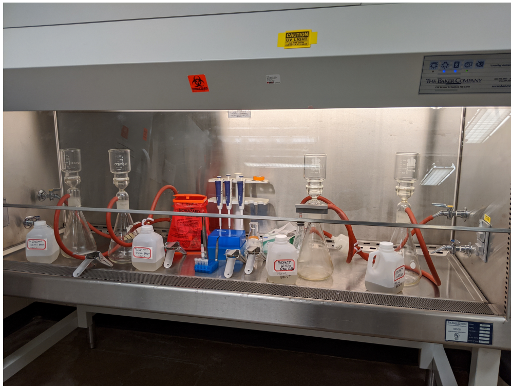
Filtration columns and bleach traps set up within the BSC.
