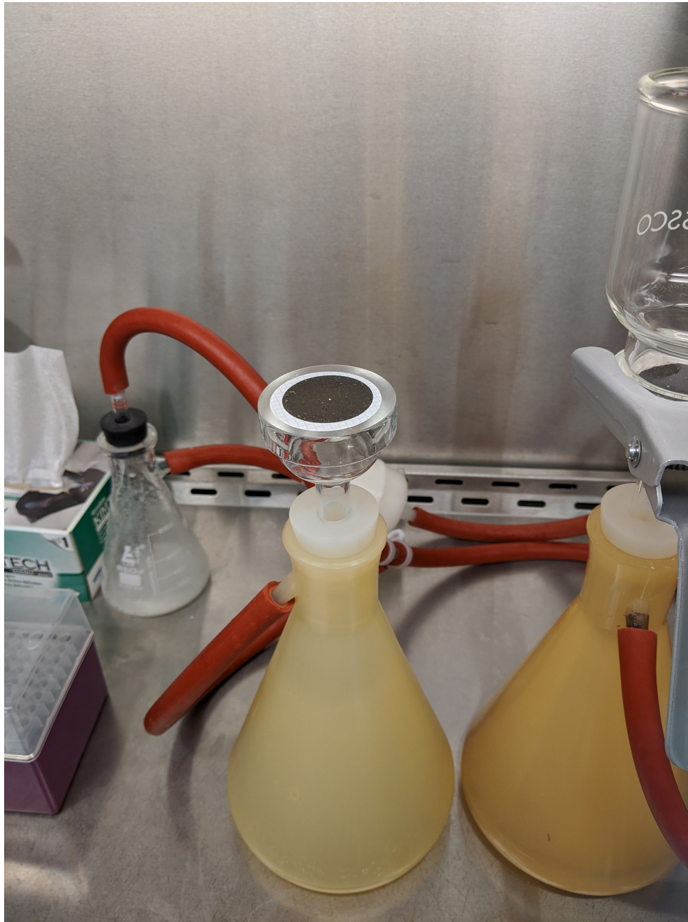
Filter with solids caked on after filtration.
