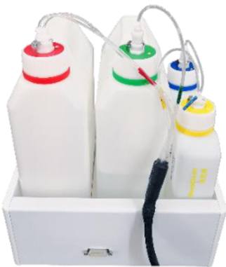
Figure 3: Reagent containers & Tubing Connections
