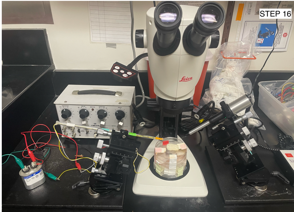
Figure 8. Full injection and electroporation set-up with clay tadpole platform positioned under dissection microscope
