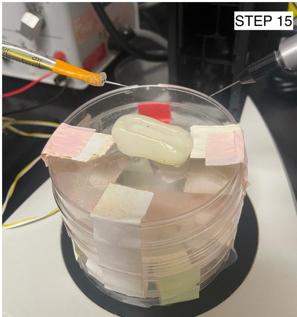
Figure 7. Hill-shaped bed mounted on top of Petri dishes to hold tadpoles
