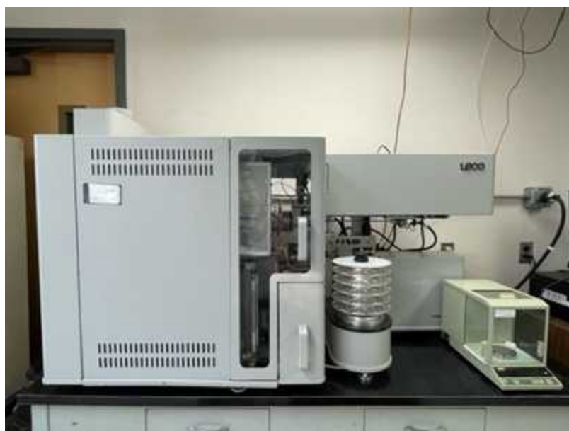
Figure 2. Leco instrument for the use of high-temperature combustion to measure the C and N contents of samples. Photograph by Michel Cavigelli.
