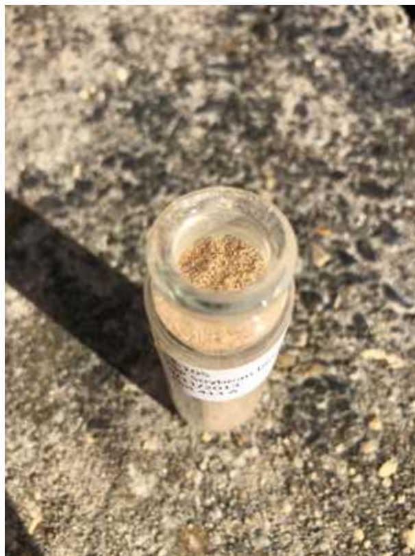
Figure 1. Soybean tissue subsample ground to \leq 1 mm in an archive container with the lid removed. Photograph by Michel Cavigelli.
