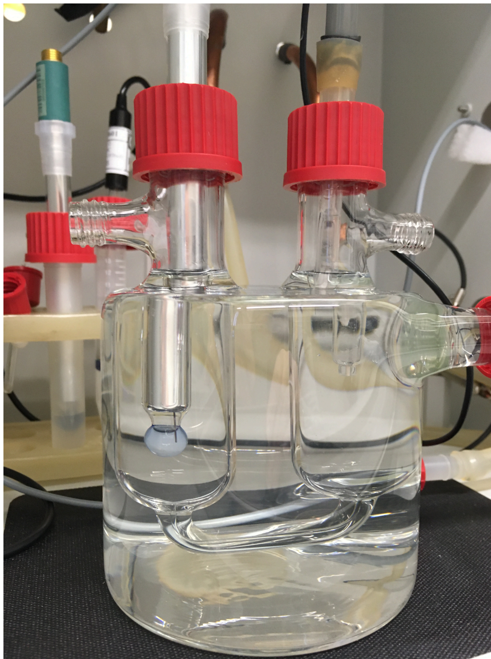
Special water-jacketed glass cell from Gebr. Rettberg.
