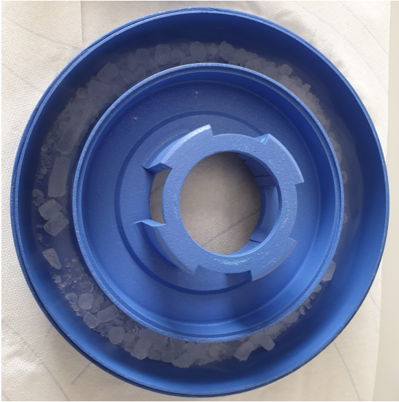
The bottom part of a CoolPrep FastPrep adaptor filled with a recommended amount of dry ice.
