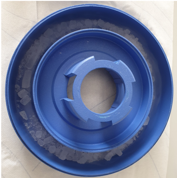
The bottom part of a CoolPrep FastPrep adaptor filled with the recommended amount of dry ice.
