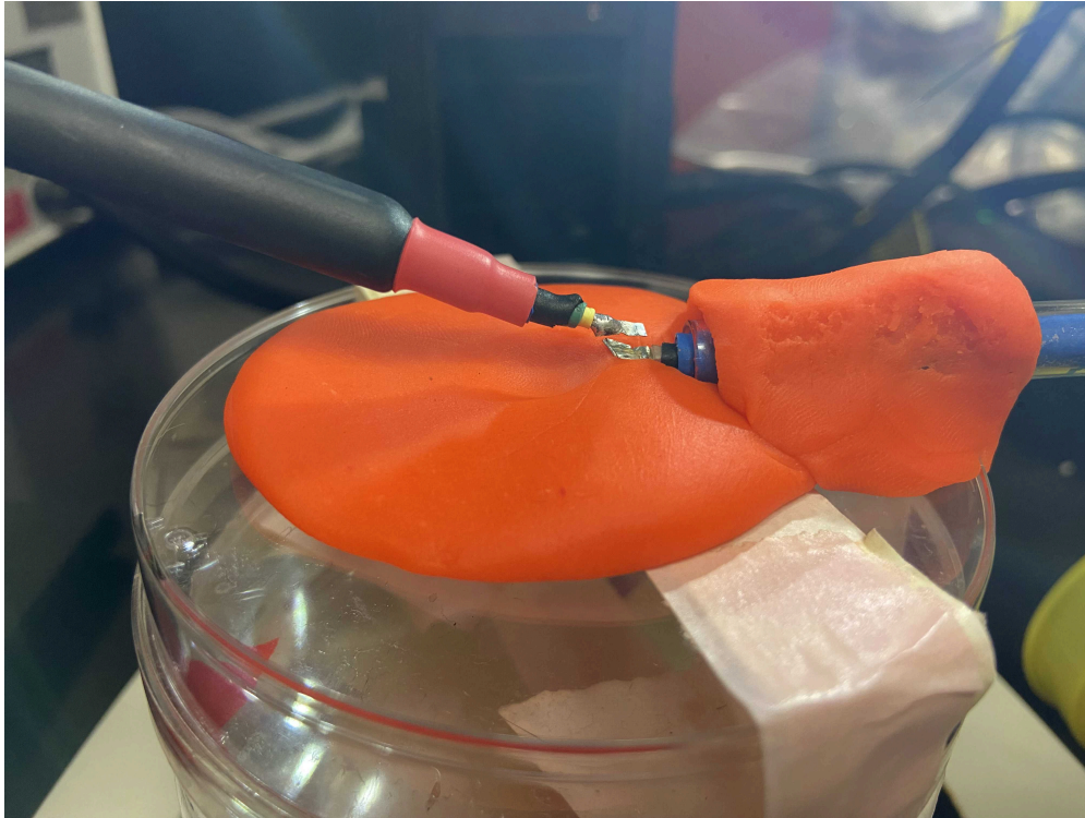
Figure 2. A cathode mounted on a micromanipulator in position to make contact directly above the anode during the electroporation procedure.
