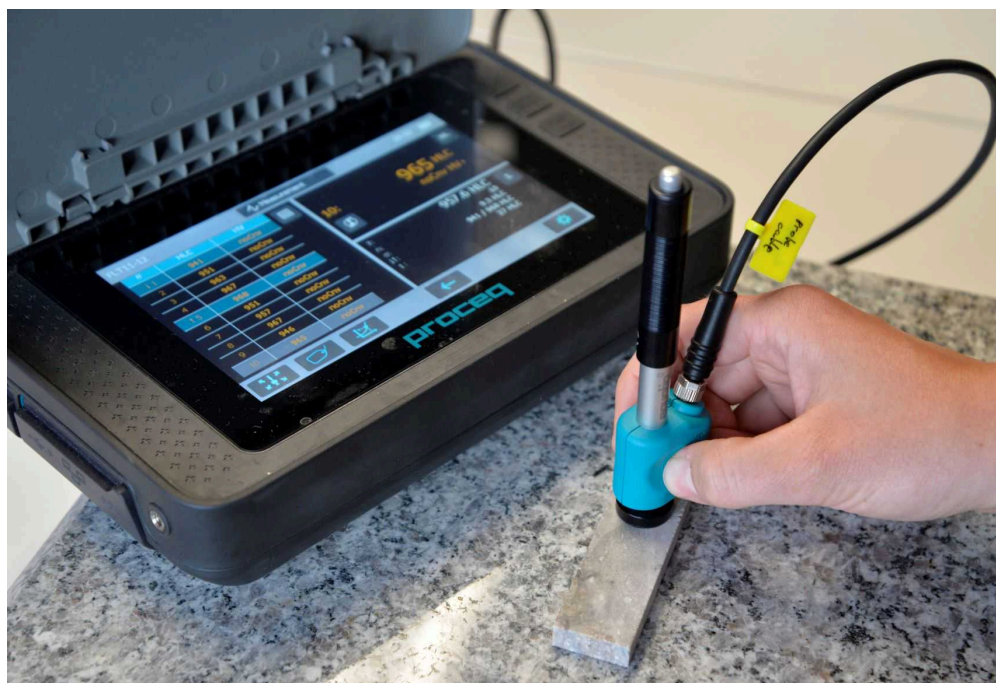
Measuring Leeb rebound hardness.
