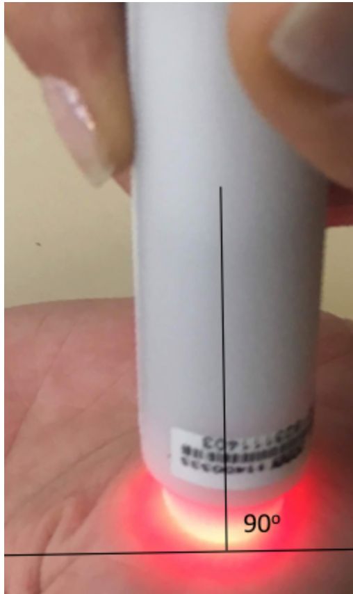
Figure 2 - Axis of the sensor when touching the skin
