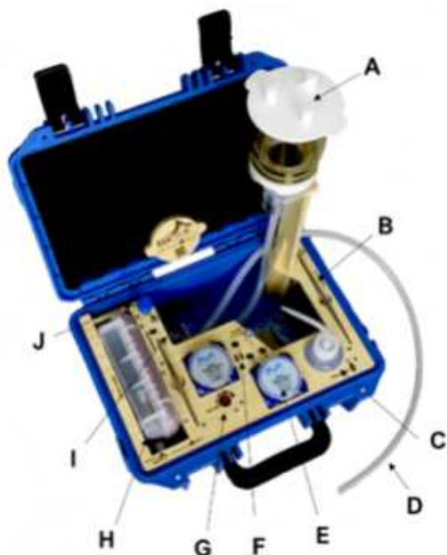
Figure 3 : Assemble the Lamprey v4.0. A) Filter holder, B) Tweezers, C) Wash bottle, D) Silicone tubing, E) Membrane, F) Tube holder, G) Potentiometer, H) Lithium battery / Waterproof box, I) Peristaltic pump, J) Bleach tube
