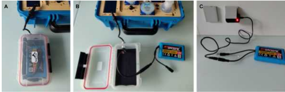
Figure 6 : Battery connection. A) Waterproof box, B) battery connected to the pump, C) Battery in charge
