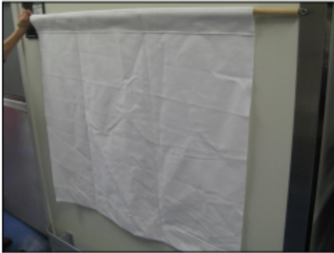
Figure 4: Ticks drag construction.
