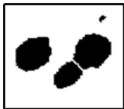
Fig. 19. A magnified portion of Fig. 16 after the Watershed has been applied showing the 1-pixel width line placed between adjacent cells.
