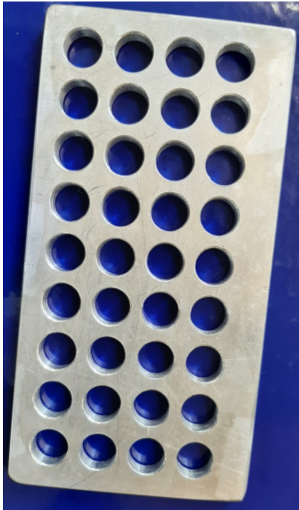
Aluminium cylindrical moulds (1.1 cm diameter and 0.6 cm height)
