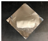
A-6. Wrap the cheesecloth with aluminum foil for sterilization by autoclave (per individual organization's protocol).
