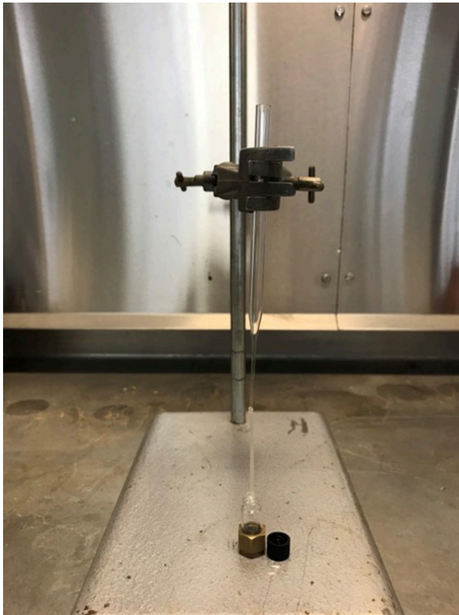
Set-up for eluting PDMS tube using Pasteur pipette
