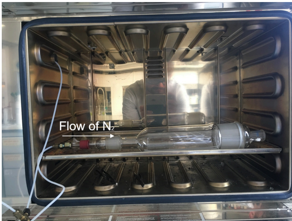
Modified heating oven containing glass vessel with pre-soaked PDMS tubing, under a constant stream of nitrogen.
