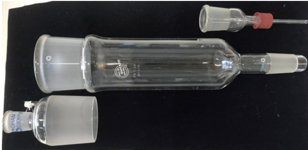
Glass vessel components used for conditioning PDMS tubing in modified oven.
