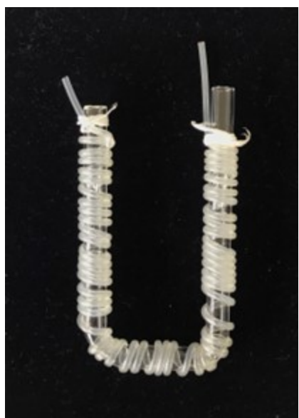
PDMS probe design: 130 cm of PDMS tubing coiled around a 19 cm hollow glass tube, bent into a U shape.
