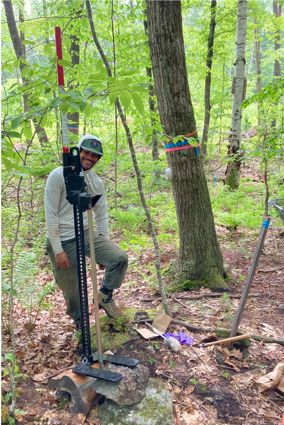
AMS Bigfoot Jack in action. We do not advise getting a core stuck with the extension pole higher than the maximum jack height.
