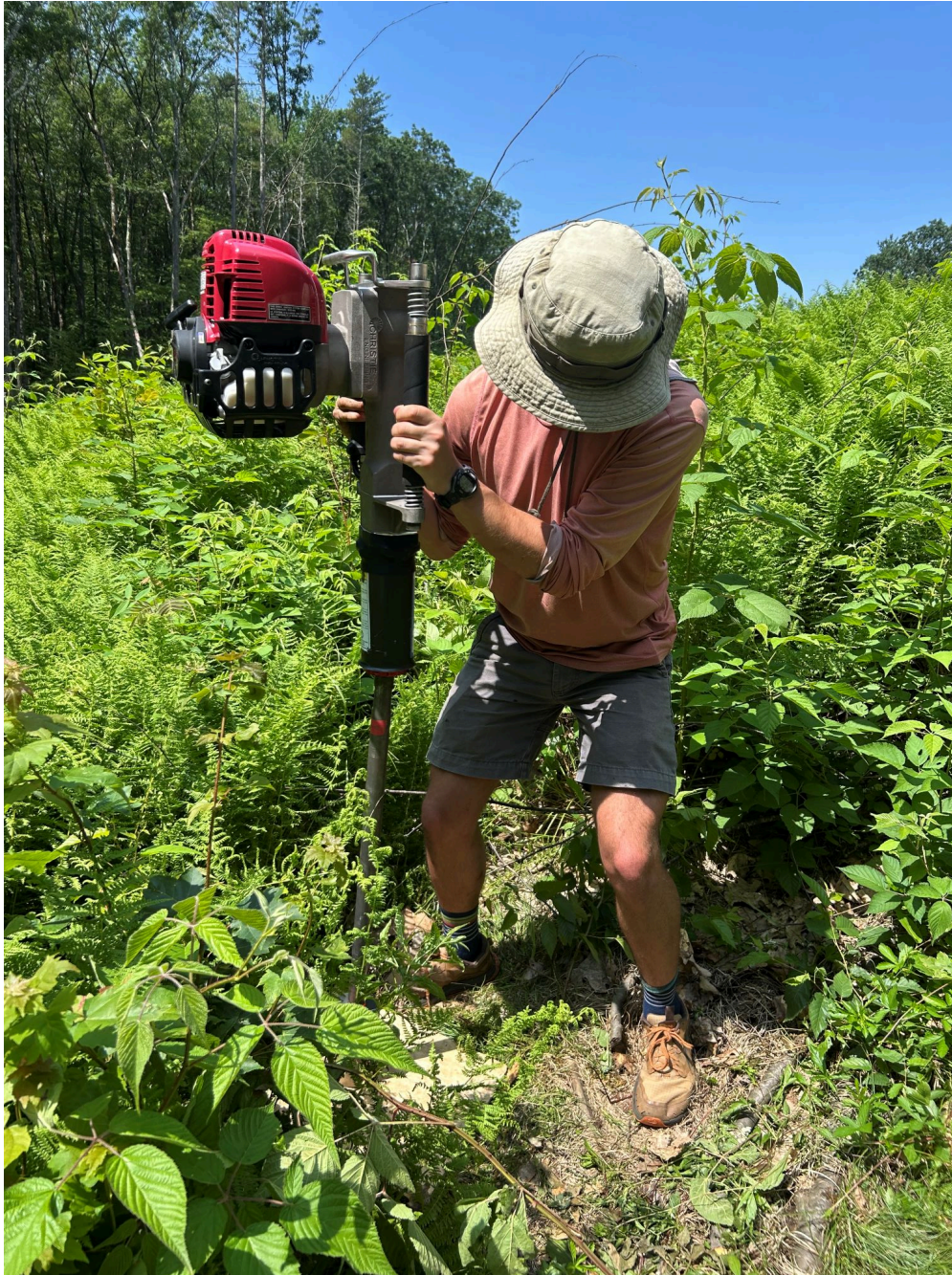
Coring with post driver.
