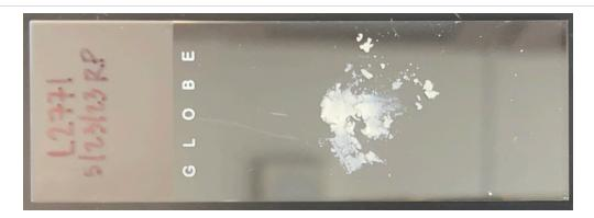
4 Using a needle tool, break up any clumps created by the metal spatula. Use it also to gather the sample towards the middle of the slide.
