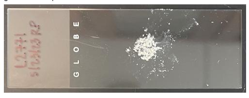
5 Immersion Oil (non-drying TYPE B) Cargille Catalog #CODE 1248 , and place ONE DROP on top of the sample.
