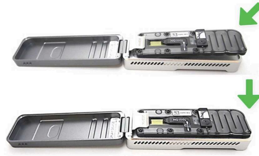
42 Slide the flow cell priming port cover clockwise to open the priming port.
