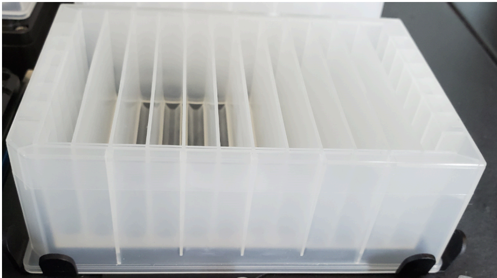
Ethanol reservoir: Used to store a large volume of ethanol.
