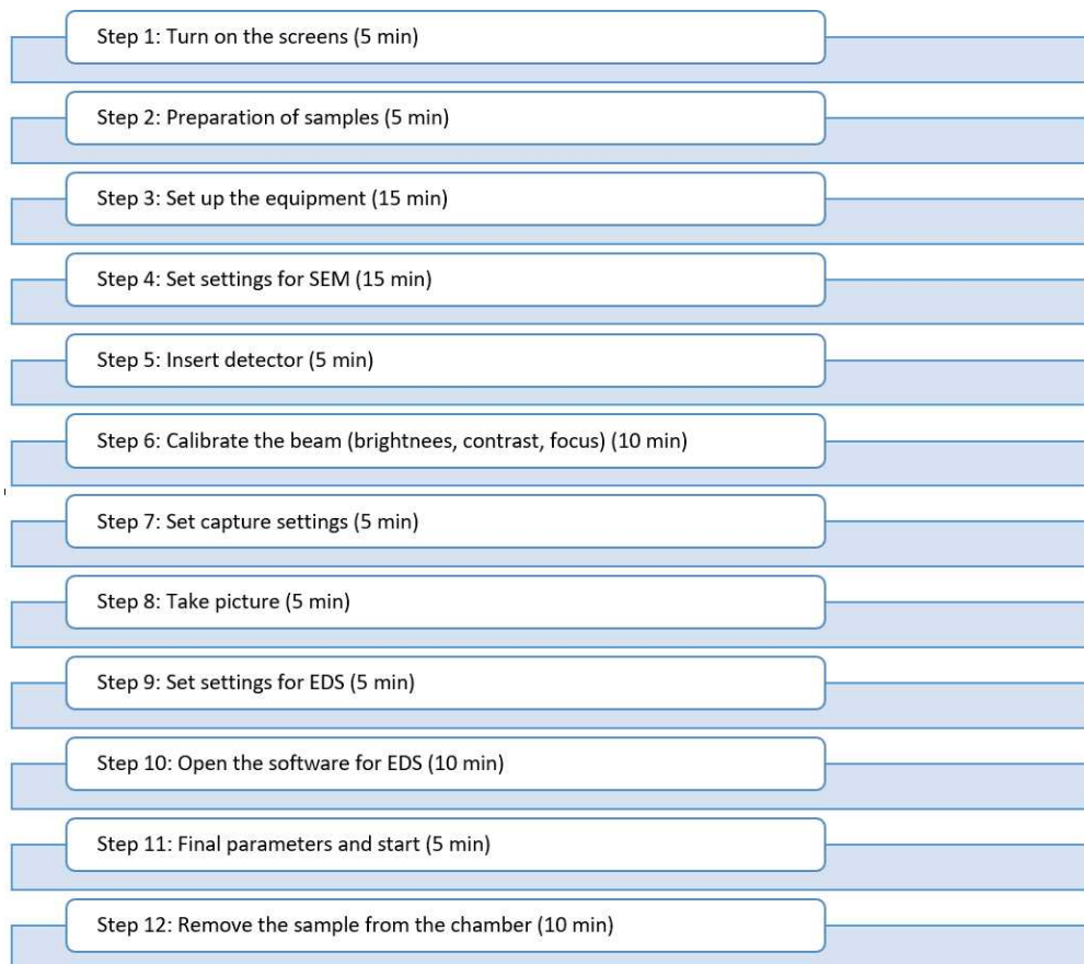
Figure 1. Diagram flow for SEM/EDS analysis
