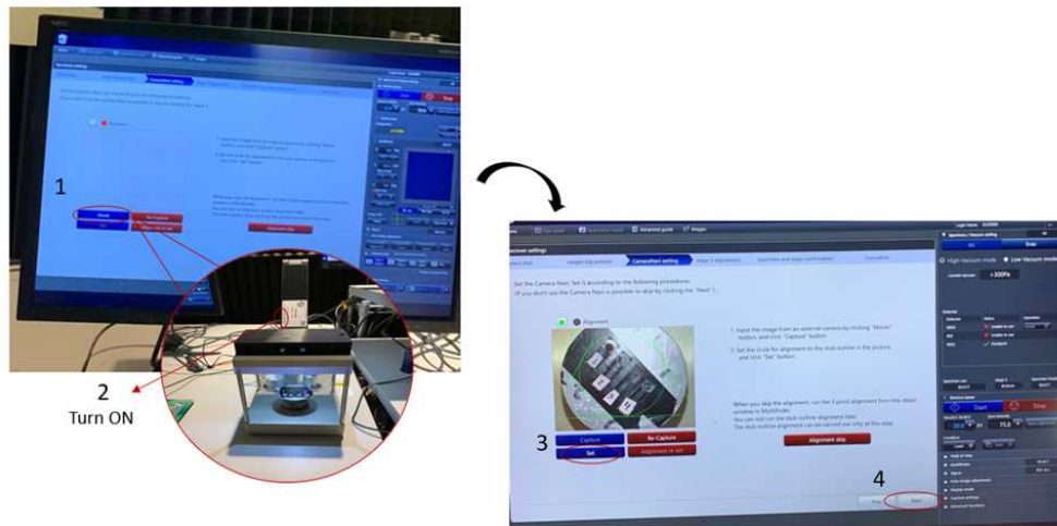
Figure 6. Place the sample holder under the camera
