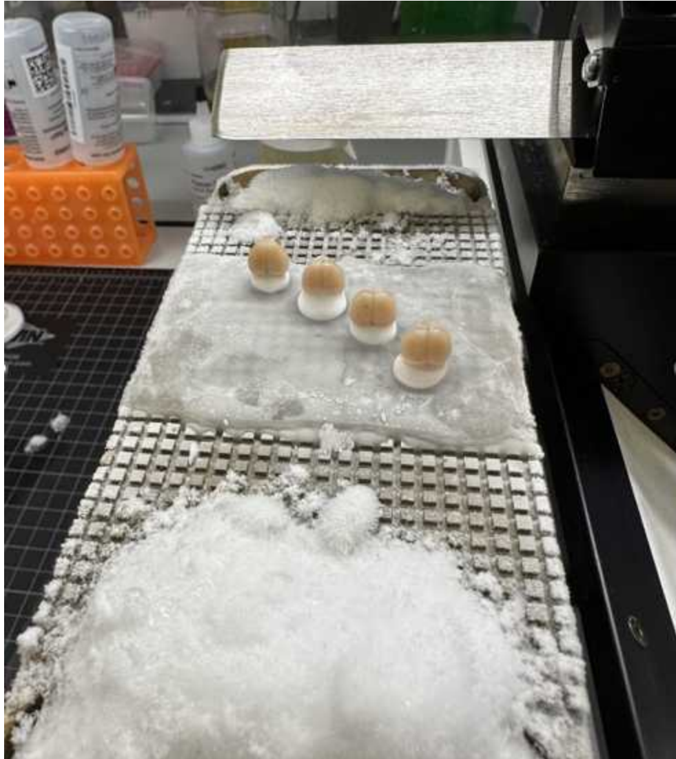
Example of 4 brains mounted in OCT in a staggered formation, with a larger 1xPBS layer that spans the entire stage.
