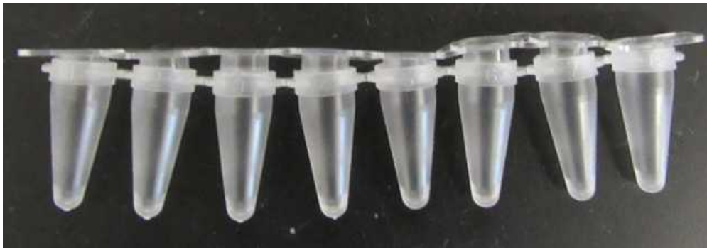
Poor seating, strip is not horizontal Lips of caps not secure inside of tubes
