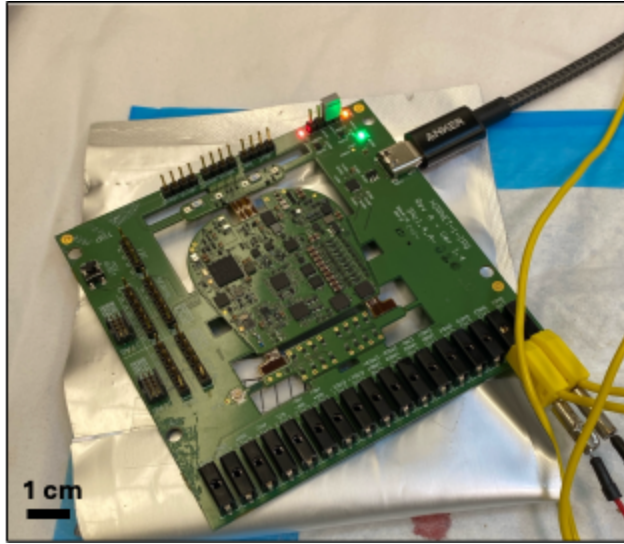
The OpenNerve stimulation board used in the study.
