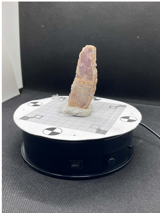
Fig. 1: Artefact on the turntable inside the light box.
