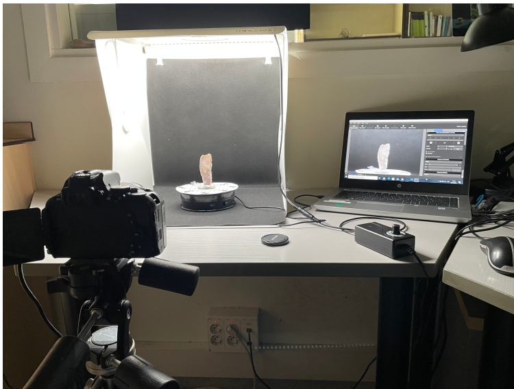
Fig. 3: Set up with the camera at a front angle, connected to the Helicon Remote .
