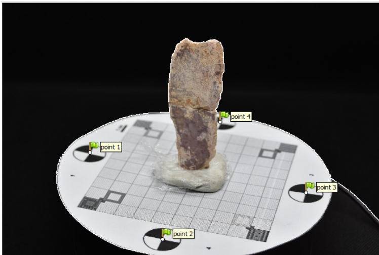
Fig. 17: The marker points use the photogrammetric scale marker as a reference.
