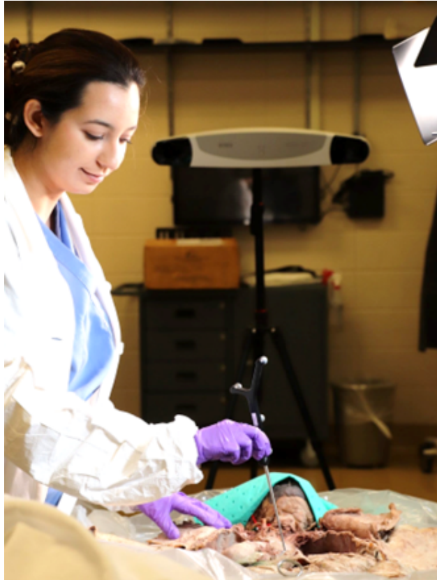
Figure 4: Photo of researcher using the stylus to trace anatomy using the NDI system sensor, seen in the background
