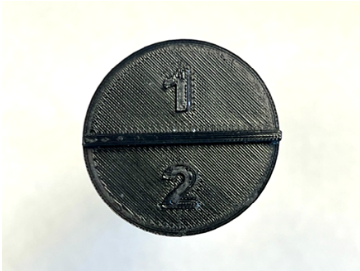
Figure 1. Custom 3D-printed cap and sample holder with sample positions labeled. Top view.
