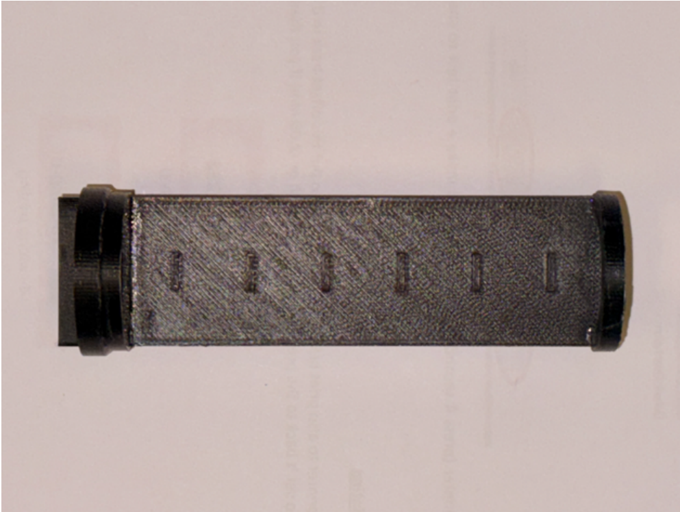
Figure 2. Custom 3D-printed cap and sample holder. Longitudinal view.
