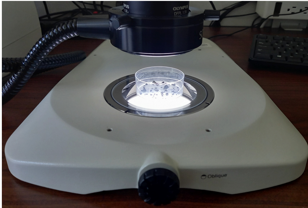
Petri dish containing charcoal fragments in transmitted light under a light stereo microscope mounted with a digital camera for image acquisition (camera not shown).
