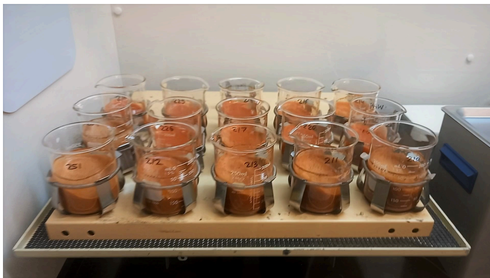
20 g soil samples in an orbital shaker reacting with 100 mL of a solution of 2.5% sodium hexametaphosphate ( \text{Na}_6\text{P}_6\text{O}_{18} ) and 5% hydrogen peroxide ( \text{H}_2\text{O}_2 ).
