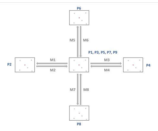
Schematic representation of the measurement scheme. The recorded positions are called one cycle of reprepeatability measurements. Only the central bead (red) will be used for the analysis. Other beads in the field of view can be tolerated as long as they have a distance of > 10  $\mu$ m from the central bead.
