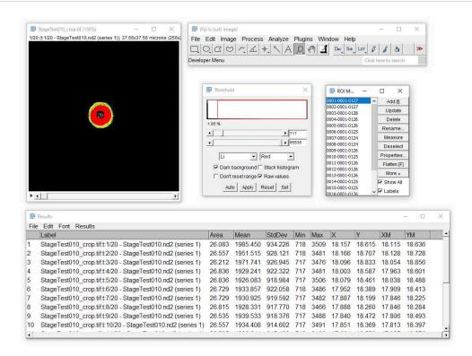
The obtained table from the "Analyze Particles" operation. To report on the stage performance, columns X, Y, XM and YM are the most relevant. The table can be saved as a ".CSV" file.
