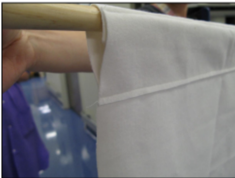
Figure 5: Details of the ticks drag construction.
