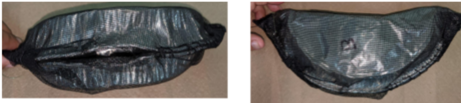
Figure A2: Leech trap, pie pan design.
