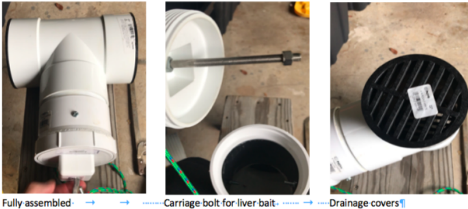
Figure A10: PVC pipe trap
