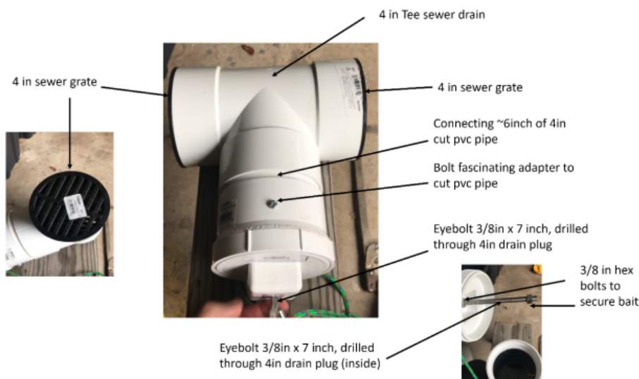
Figure A11: PVC pipe trap construction.
