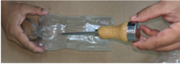
Figure A6: Holes being made with icepick.
