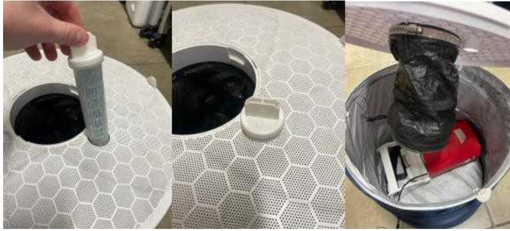
Fig. 5. The BG Lure and its correct installation in the lid of the BG Sentinel trap. Additional attractants, including dry ice (CO 2 ) can be placed inside the trap. Odors are pushed out through the perforated lid by the fan.
