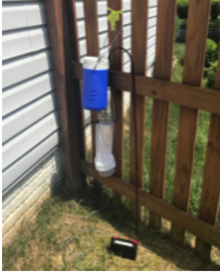
Fig. 2. If the trap cannot be hung directly from the cooler, the cooler and trap may both be hung from the hook or post. In this instance, ensure that the bottom of the cooler (where the holes for CO 2 release are located) is positioned just above the top of the trap.
