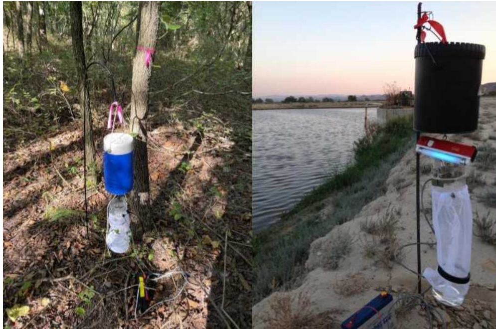
Fig. 1. CDC traps baited with dry ice coolers. In these images, the trap device is hung directly from the bottom of the cooler using a hook or D-ring that has been installed onto the cooler for this purpose.
