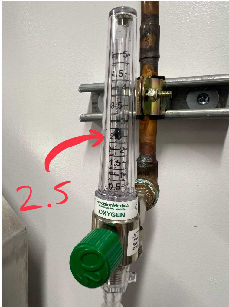
Steel bead of Oxygen Regulator is at 2.5
