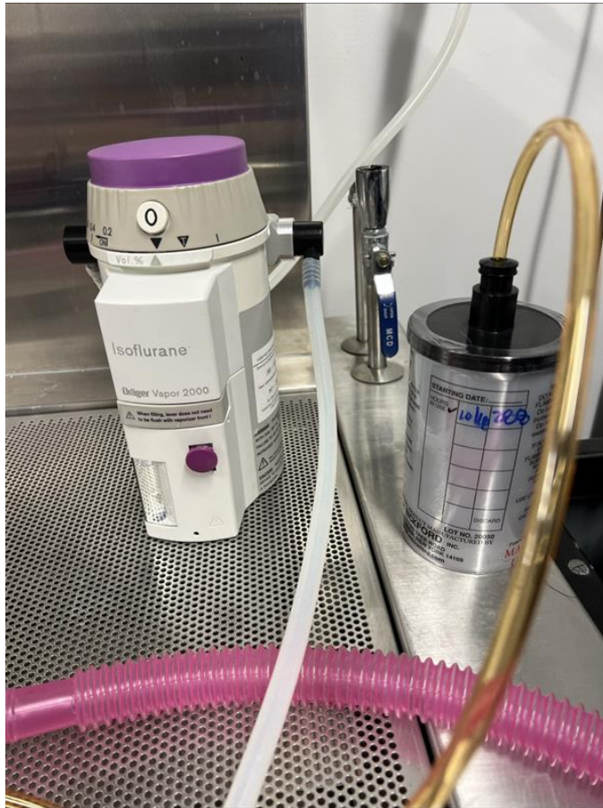
Proper configuration of the isoflurane vaporizer with the F/air canister.
