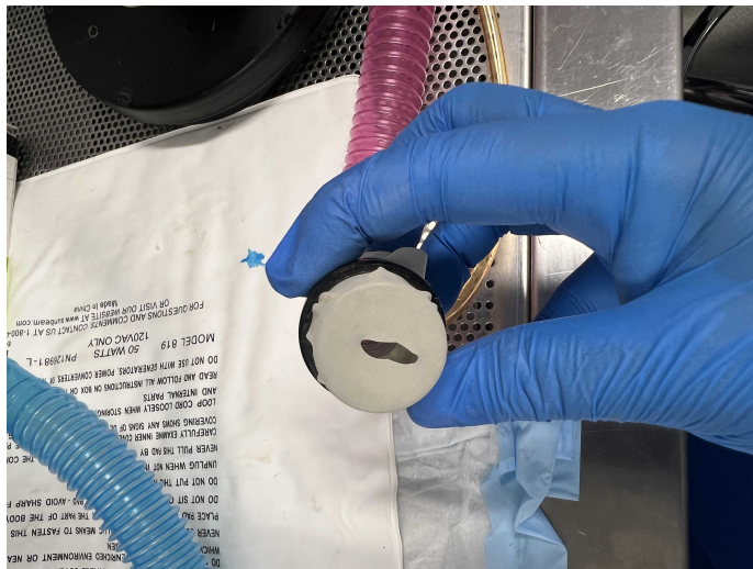
Appearance of new elastic vapor shield (with slit) on the nose cone.
