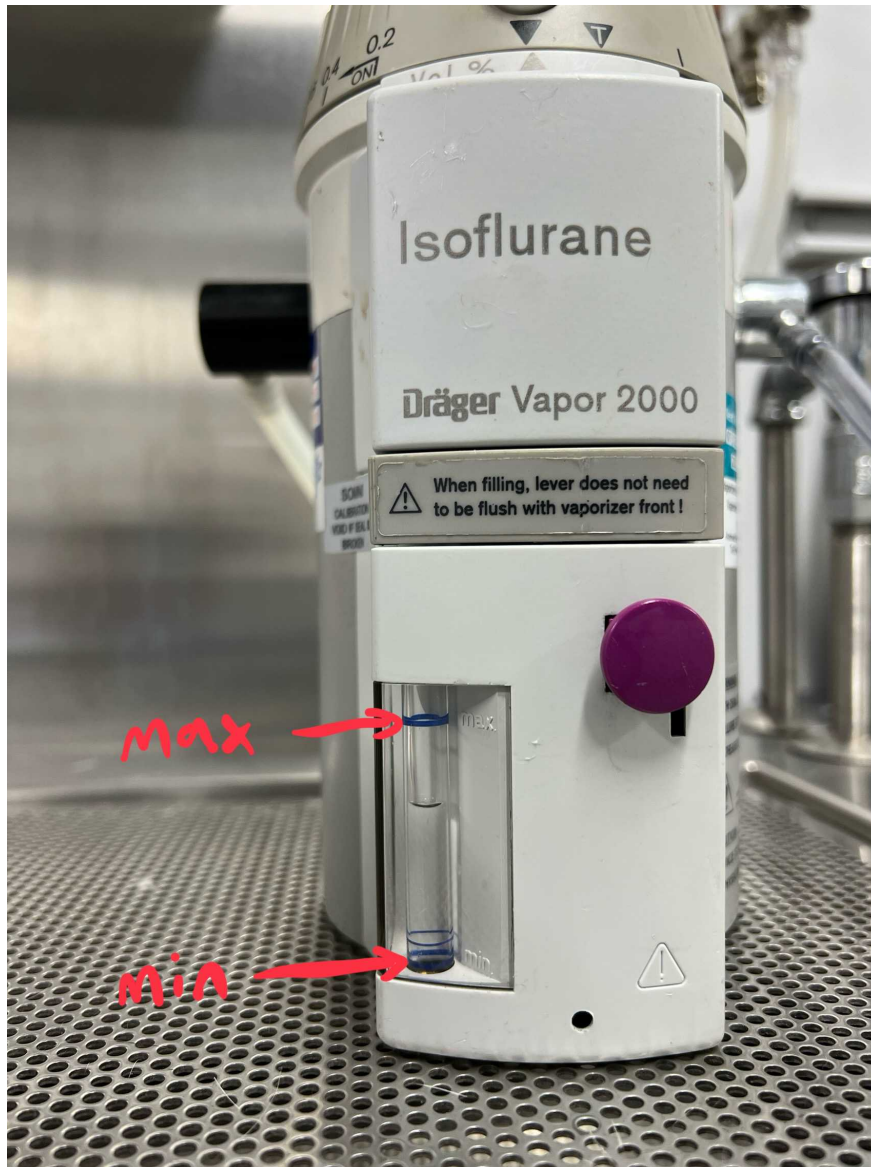
Minimum and Maximum fill lines of Dräger Vapor 2000 Isoflurane model.
