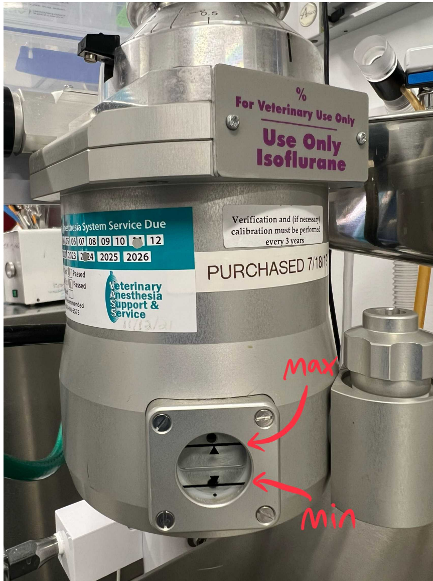
Minimum and Maximum fill lines of VIP 3000 Veterinary Vaporizer model.
