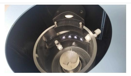
11.4 When the filter is fully saturated, and water cycle is complete, add more de-ionized water until the level is just below the top white spout.
