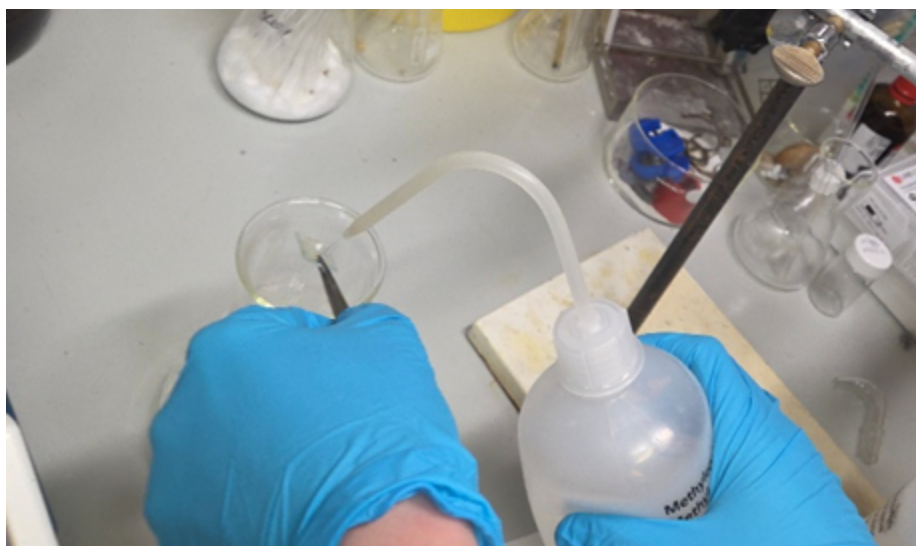
Figure 7. Step 2. quickly rinse with toluene
