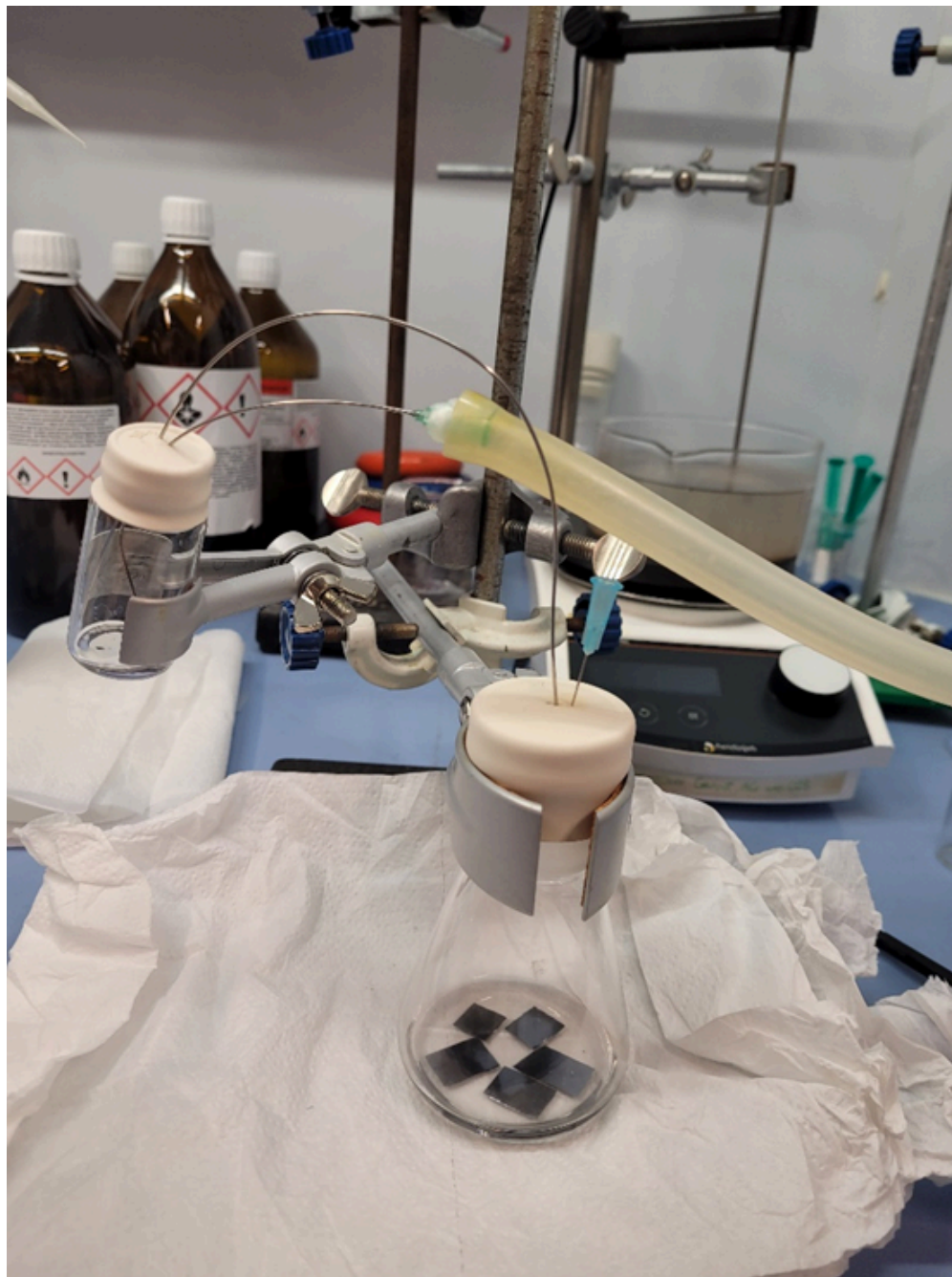
Figure 8. Proposed setup for introducing BIB for substrates modification under argon conditions
