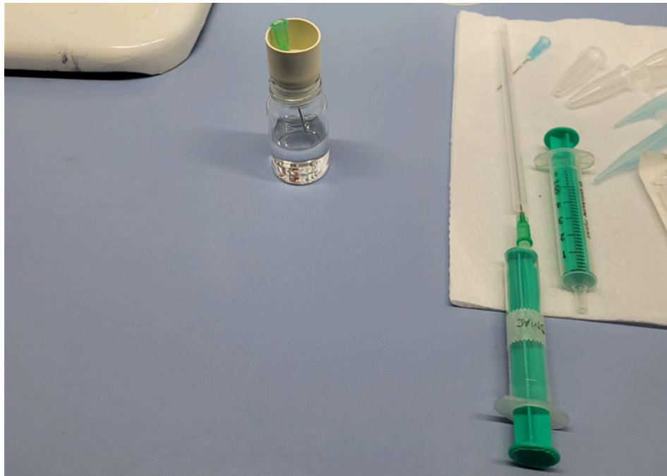
Figure 9. Setup proposed to rinse needles and cannulas
