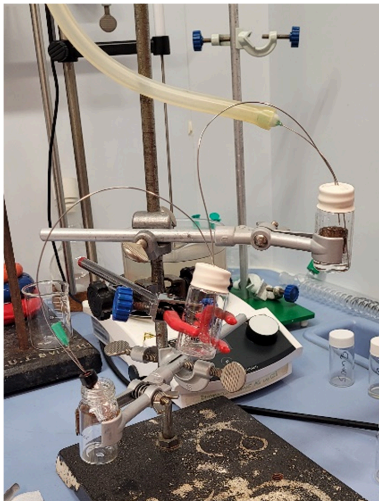
Figure 10. Setup proposed to prepare monomers and catalyst mixture under argon conditions.
