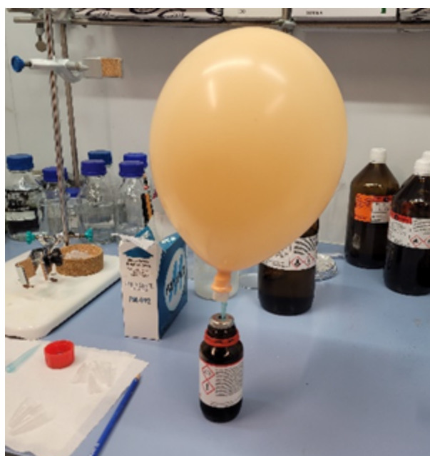
Figure 5. Setup proposed to remove APTES under argon atmosphere.
