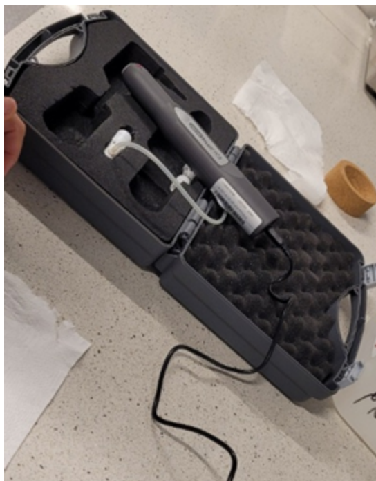
Figure 2. Piezo brush is used for plasma treatment of the surface to increase the oxidation and improve the yield of reaction for APTES monolayer formation.
