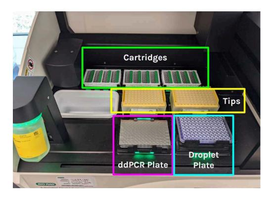
15.7 When droplet generation is done, open the lid and remove the droplet plate from the Auto DG cold block and place it in the metal carrier inside the plate sealer.
