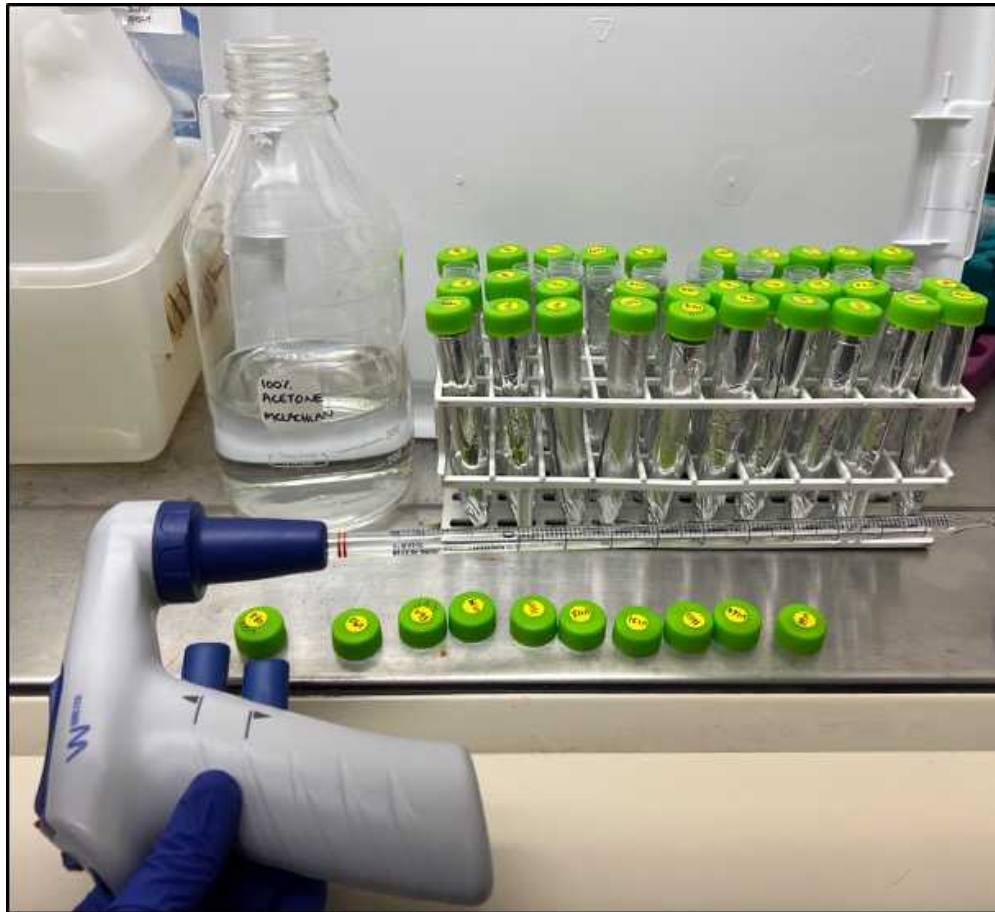
Fig. 5. Supplies needed for adding acetone to ground coral sample tubes. This step must be conducted inside a fume hood.
