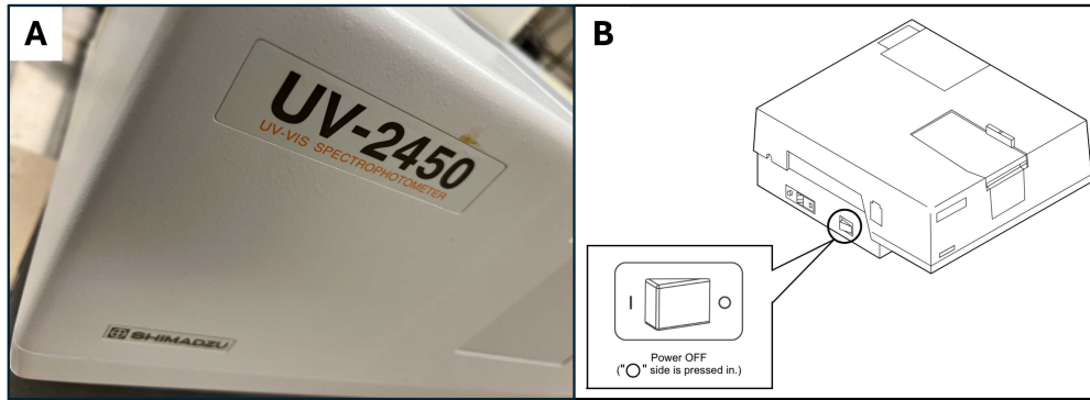
Fig. 7. A) SHIMADZU UV-VIS 2450 spectrophotometer and B) labeled diagram showing the location of power switch (image source: UV-VIS 2450 manual).
