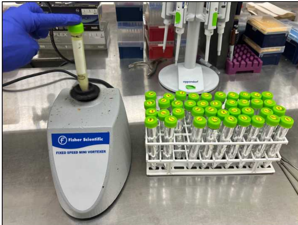
Fig. 6. Vortex sample tubes to ensure that the ground coral material mixes thoroughly with the acetone.
