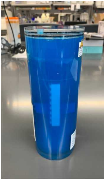
Geometric phantom (radius = 35 mm and height = 190 mm)
