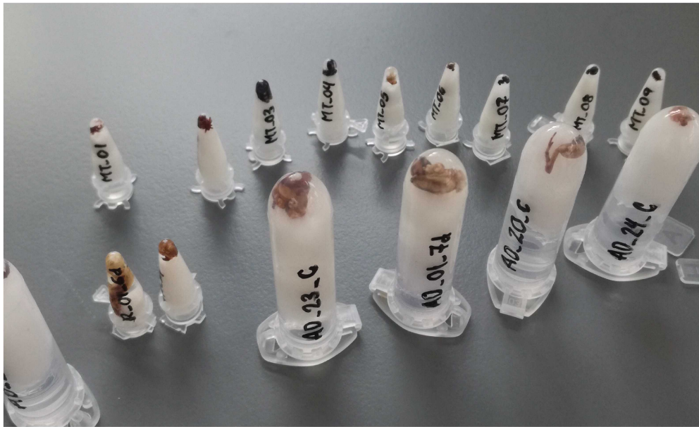
Figure 2. The selection of the tube will depend on the size of the actual specimen and the capabilities of the scanner. A larger working distance allows more freedom in the width of the tube. A shorter working distance requires a smaller tube to get as close as possible to the specimen.
