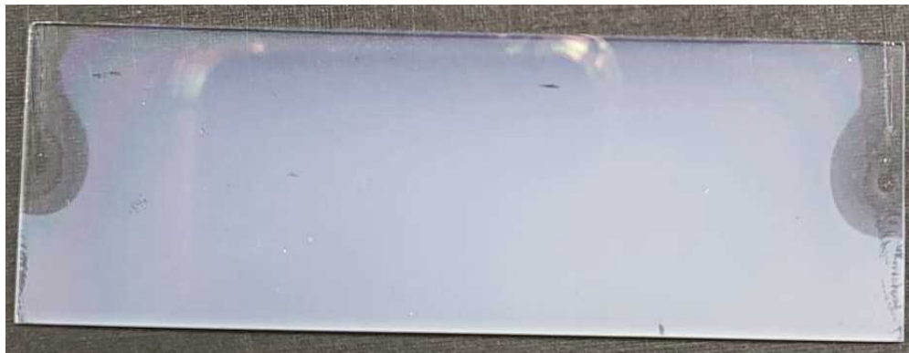
\alpha -Cyano-4-hydroxycinnamic acid (CHCA) matrix applied to a glass slide by sublimation.
