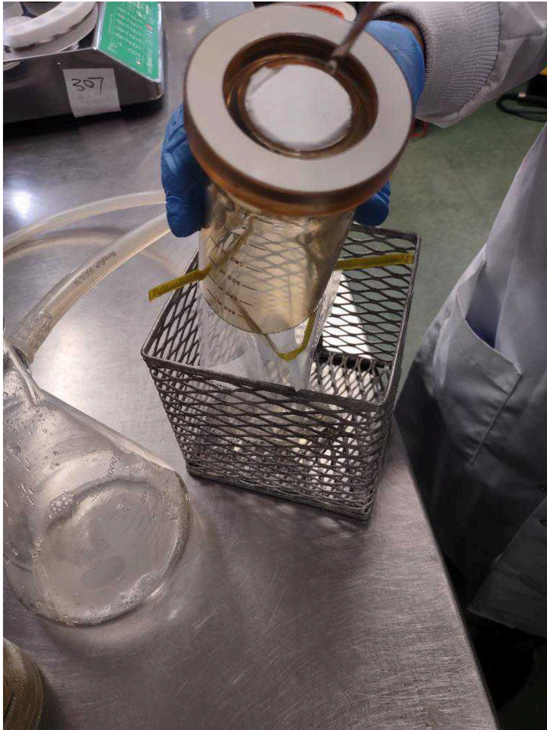
Magnetic funnel containing 47 mm glass fiber filter is separated from base, inverted, and sterile forceps are used to nudge or poke glass fiber filter (filtercake) into sterile Whirl-Pak bag.
