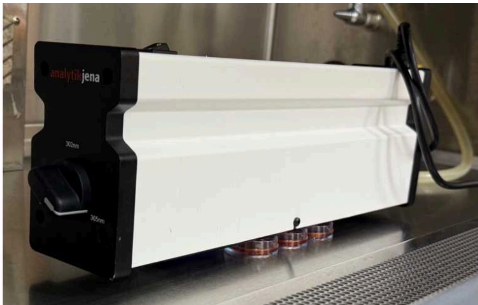
Figure 17. Gels exposed to 365 nm UV light with diluted sulfo-SANPAH solution, binding SANPAH to the gel surface and enabling subsequent collagen cross-linking.
