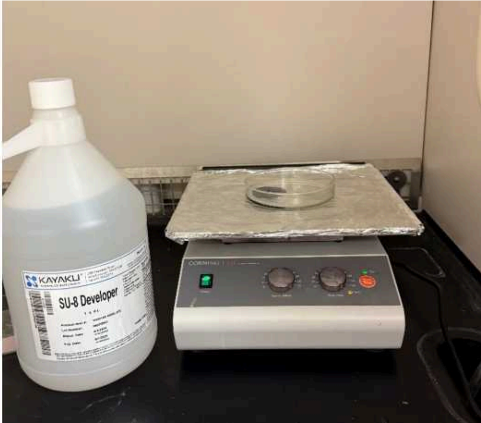
Figure 8. Silicon wafer developing in SU-8 developer solution on shaker plate.
