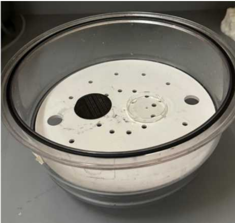
Figure 10. Wafer and (TRIDECAFLUORO-1,1,2,2-TETRAHYDROOCTYL) SILANE filled petri dish in desiccator chamber.
