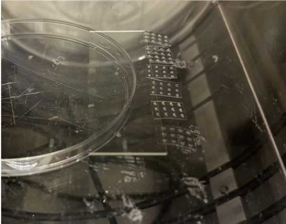
Figure 13. PDMS masks placed on the edge of a glass microscope slide elevated by a petri dish for O 2 plasma treatment.
