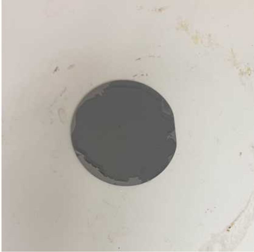
Figure 5. Image of SU-8 after spreading it on a silicon wafer using a razor blade.
