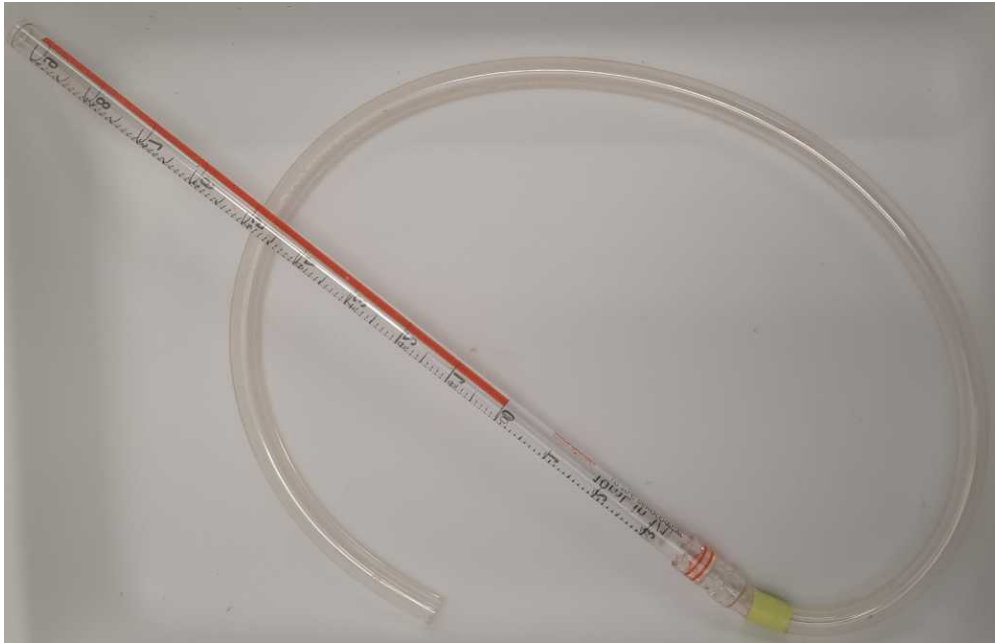
Figure 1. Aspirator tool for collecting mosquitoes.
