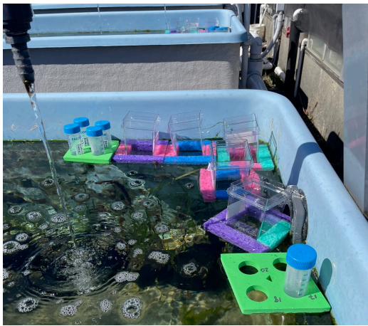
Image 4. Example of how the milking chambers (magenta boxes and 50 mL conical tubes) look in their respective floats in the tank. Thank you to Sogin Lab member Diane-Marie Branche-Smith for the photo.
