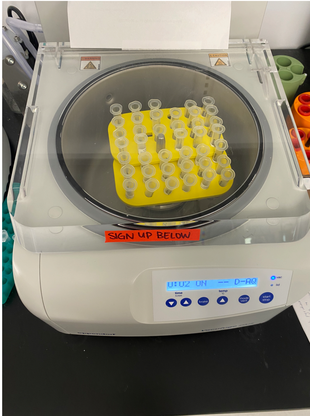
Image 4: Set up of microtube floats loaded with PPL columns in the vacuum concentrator for drying
