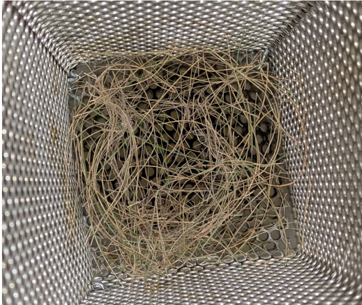
Figure 2: Grass samples placed within the metallic mesh container before combustion
