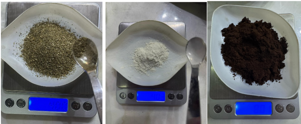
weighing dry components, dried remains of yerba mate, sodium alginate, dried coffee grounds
